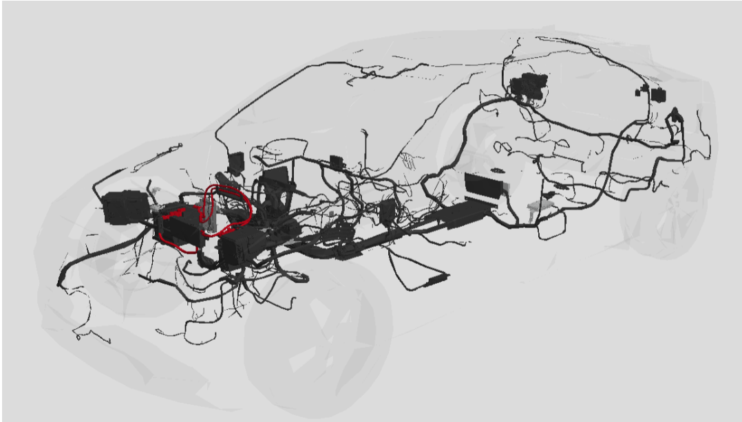
Figure 3 - Three-dimensional schematic of the wiring of the car model.
