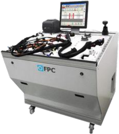
Figure 23 - Wire harness test board. Retrieved from: https://www.fpc.cz/wire-harness-testing/ [73]
